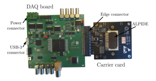
Figure 4.1: Picture of the setup used for the tests of the full-scale ALPIDE prototypes.
