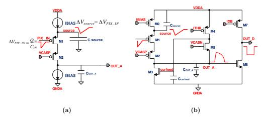
Figure 3.9: Schematic drawing of the input branch the analog front-end (a) and of the concept of the analog front-end (b). Adapted from Ref. [61].
