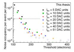
**Figure 5.29:** Dependency of the noise occupancy on  $I_{thr}$  at  $V_{BB} = -1$  V for sector 2 of chip W6-14 after masking the 20 noisiest pixels. The dotted line at  $10^{-6}$  hits/event/pixel represents the upper limit acceptable for the upgrade.
