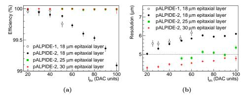
**Figure 5.40:** Comparison of the detection efficiency (a) and resolution (b) of the pALPIDE-1 and pALPIDE-2 for the sectors with a PMOS reset and 4  $\mu$ m spacing between the collection n-well and the surrounding p-well at  $V_{BB} = -6$  V and  $V_{CASN} = 160$  DAC units. Points for the pALPIDE-2 are taken from Ref. [59].
