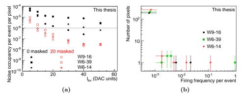
Figure 5.33: In panel (a) the noise occupancy values of three chips at  $V_{BB} = -3 \text{ V}$  and  $V_{CASN} = 135 \text{ DAC}$  units is plotted as a function  $I_{thr}$  without masking any pixels and after masking the 20 noisiest pixels. Panel (b) shows the number of pixels firing with a certain firing frequency per event for the same three chips at  $V_{BB} = -3 \text{ V}$ ,  $I_{thr} = 40 \text{ DAC}$  units and  $V_{CASN} = 135 \text{ DAC}$  units without masking any pixels.
