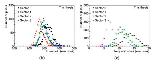
**Figure 5.1:** Panel (a) shows an example of the fit to the firing probability of one pixel of chip W2-31 at  $V_{BB} = 0$  V,  $I_{thr} = 60$  DAC units and  $V_{CASN} = 57$  DAC units. Panels (b) and (c) show the threshold and noise distribution respectively of the different pixels of the sensor at the same settings.
