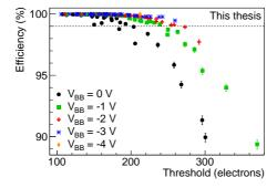
**Figure 5.7:** Comparison of the detection efficiency with different reverse-substrate-bias voltages for chip W9-16.
