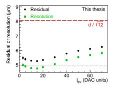
Figure 5.21: Example of the residual before the subtraction of the tracking uncertainty and the resolution after subtraction for sector 2 of chip W2-31 at  $V_{BB}=0$  V and  $V_{CASN}=57$  DAC units. The dotted line at 5  $\mu$ m represents the upper limit acceptable for the upgrade, while the dashed line around 8  $\mu$ m is the theoretical resolution in the case when only one pixel fires for each crossing particle  $(d/\sqrt{12})$ , where d=28  $\mu$ m is the pixel pitch).
