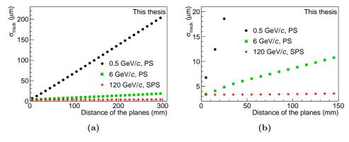
**Figure 4.8:** Panel (a) shows the comparison of the pointing resolution for different momenta, while (b) is a zoomed view showing the difference between the 6 GeV/c and the 120 GeV/c case.
