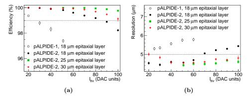
**Figure 5.41:** Comparison of the detection's efficiency (a) and resolution (b) of the pALPIDE-1 and pALPIDE-2 for the sectors with a PMOS reset and 2  $\mu$ m spacing between the collection n-well and the surrounding p-well at  $V_{BB} = -6$  V and  $V_{CASN} = 160$  DAC units. Points for the pALPIDE-2 are taken from Ref. [59].
