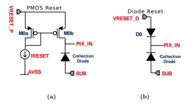
**Figure 3.12:** The two figures show the two types of reset mechanisms, which are present in the pALPIDE-1 chip: panel (a) shows the PMOS reset and panel (b) the diode reset. Adapted from Ref. [61].
