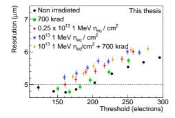
**Figure 5.26:** Comparison of resolution values for different levels of irradiation for five sensors at  $V_{BB} = 0 \ V$ .
