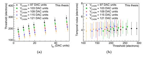
**Figure 5.2:** Measured threshold (a) and temporal noise (b) values for sector 2 of chip W9-16 at  $V_{BB} = -2$  V. The error bars show the RMS of the distributions, indicating the pixel-to-pixel fluctuations. The points in (a) are slightly shifted on the horizontal axis for better visibility.
