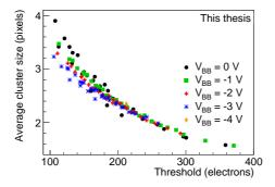
**Figure 5.16:** Comparison of the average cluster size with different reverse-substrate-bias values for chip W9-16.
