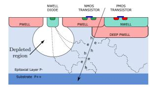
Figure 3.3: Schematic drawing of a pixel in the TowerJazz technology [45].
