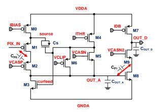
Figure 3.14: The schematic drawing of the analog front-end of the pALPIDE-3 chip [61].
