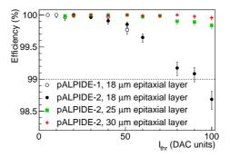
**Figure 5.42:** Comparison of the detection efficiency of sector 2 of the pALPIDE-1 (diode reset, 2  $\mu$ m spacing) and sector 3 of the pALPIDE-2 (diode reset, 4  $\mu$ m spacing) at  $V_{BB} = -3$  V and  $V_{CASN} = 135$  DAC units. Points for the pALPIDE-2 are taken from Ref. [74].
