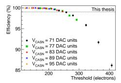
**Figure 5.3:** Detection efficiency as a function of the threshold for different  $V_{CASN}$  values for sector 2 of chip W6-14 at  $V_{BB} = -1$  V. The dotted line at 99% represent the minimum requirement for the upgrade.
