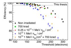
**Figure 5.8:** Comparison of the detection efficiency with different irradiation levels for five sensors at  $V_{BB} = 0$  V.
