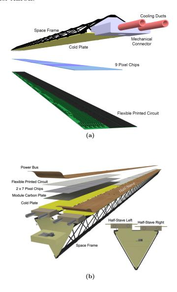
**Figure 3.2:** Schematic drawing of (a) the Inner Barrel stave and (b) the Outer Barrel stave, adopted from Ref. [45].
