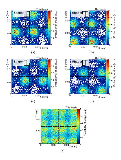
**Figure 5.39:** Probability of the appearance of three-pixel clusters with the shape of the letter **L** within two times two pixels as a function of the impinging point of the track at  $V_{BB} = 0$  V,  $I_{thr} = 20$  DAC units and  $V_{CASN} = 57$  DAC units for chip W2-25. Panels (a), (b), (c) and (d) show separately the four possible rotations indicated on the plot, while (e) shows the four rotations summed up.
