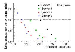
**Figure 5.32:** Comparison of the noise occupancy values for the different sectors of chip W9-16 after masking of the 20 noisiest pixels at  $V_{BB} = -3$  V and  $V_{CASN} = 135$  DAC units.
