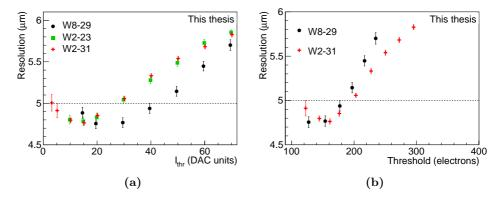
**Figure 5.24:** Resolution values for the different chips at  $V_{BB} = 0$  V and  $V_{CASN} = 57$  DAC units as a function of  $I_{thr}$  (a) and the threshold (b) for those sensors where the threshold has been determined.
