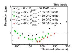
**Figure 5.25:** Resolution values for chip W2-31 comparing different reverse-substrate-bias values.
