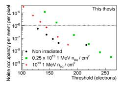
**Figure 5.34:** Comparison of the noise occupancy values after masking the noisiest 20 pixels with different irradiation levels for three sensors at  $V_{BB}=-3~{\rm V}$  and  $V_{CASN}=135~{\rm DAC}$  units.
