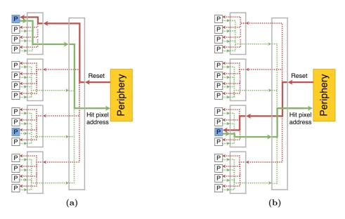
**Figure 3.6:** Schematic drawing of the principle of operation of the readout and reset of the pixels by the AERD.
