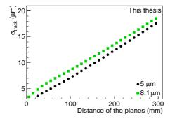
**Figure 4.11:** Effect of the resolution of the tracking planes on the pointing resolution of the track at the DUT.
