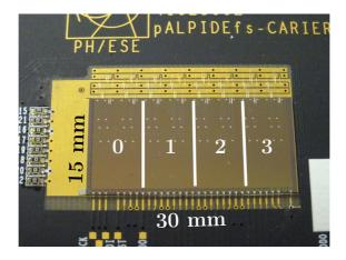
Figure 3.11: Picture of the pALPIDE-1 chip with the four sectors indicated.
