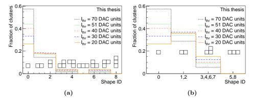
**Figure 5.36:** Both plots show the fraction of clusters with certain shapes at  $V_{BB} = 0$  V and  $V_{CASN} = 57$  DAC units for chip W2-25. In (a) each bin corresponds to a rotation of a shape, while in (b) each bin correspond to a shape with all rotation included. The shapes are indicated by drawings for each ID.
