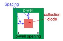
Figure 3.5: Illustration of the spacing between the collection diode and the surrounding p-well.
