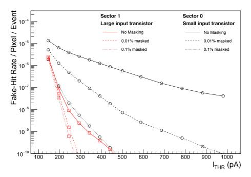
**Figure 5.43:** Comparison of the noise occupancy values for sector 0 (small input transistor) and sector 1 (optimized input transistor) of the pALPIDE-2 at  $V_{BB} = -3 \text{ V}$  and  $V_{CASN} = 135 \text{ DAC}$  units [59].
