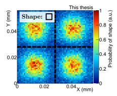
**Figure 5.37:** Probability of the appearance of one-pixel clusters within two times two pixels as a function of the impinging point of the track at  $V_{BB} = 0$  V,  $I_{thr} = 20$  DAC units and  $V_{CASN} = 57$  DAC units for chip W2-25.
