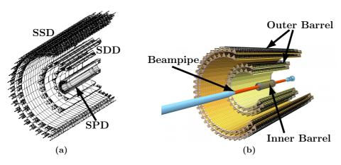
Figure 3.1: Panel (a) shows the layout of the current ITS [47], while (b) shows the layout of the upgraded ITS [45].
