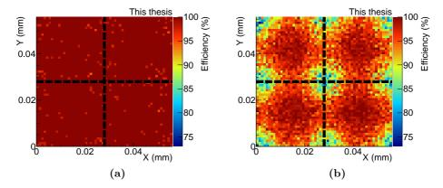
**Figure 5.9:** Detection efficiency as a function of the impinging point of the track within the smallest repeated unit of the chip (two times two pixels) at  $V_{BB} = 0$  V and  $V_{CASN} = 57$  DAC units for chip W2-25. Panel (a) shows the efficiency in the case of a low threshold ( $I_{thr} = 20$  DAC units), while (b) shows the same in the case of a high threshold value ( $I_{thr} = 70$  DAC units).
