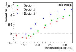
**Figure 5.23:** Comparison of the resolution of the different sectors of chip W2-31 at  $V_{BB} = 0 \text{ V}$ .
