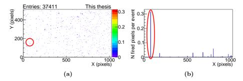
Figure 5.28: Panel (a) shows a typical hit map of a run without an external source at  $V_{BB} = -3$  V with  $I_{thr} = 30$  DAC units and  $V_{CASN} = 135$  DAC units from the chip W9-16 with the firing frequency of the pixels indicated by the color code. Panel (b) shows the projection of the same hit map to the x-axis. In this case the y-axis corresponds to the average number of pixels firing in each column. The same very noisy pixel is highlighted in both plots.
