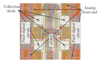
**Figure 3.13:** The routing plan of the smallest repeated unit of two times two pixels  $(56 \ \mu\text{m} \times 56 \ \mu\text{m})$  with the different areas indicated [62].
