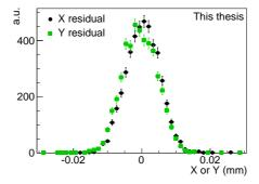
**Figure 5.20:** Example of the residual distribution for sector 2 of chip W2-31 at  $V_{BB} = -3$  V,  $I_{thr} = 30$  DAC units and  $V_{CASN} = 135$  DAC units.
