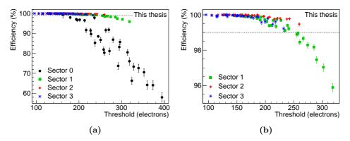
**Figure 5.4:** Comparison of the detection efficiency between the different sectors for chip W9-16 as a function of the threshold at  $V_{BB} = -3$  V. Panel (a) shows all four sectors, while (b) is a zoom without sector 0 to show the difference between sectors 1 to 3.
