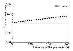
Figure 4.7: Ratio of the pointing resolution if there is air or vacuum between the layers.
