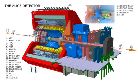
Figure 2.1: Schematic drawing of the ALICE detector [44].
