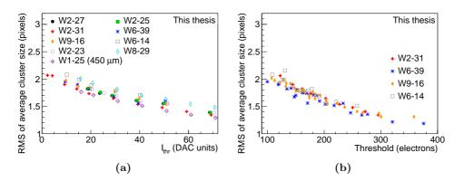
**Figure 5.14:** Panel (a) shows the chip-to-chip fluctuation of the RMS of the average cluster size as a function of  $I_{thr}$  at  $V_{BB} = 0$  V and  $V_{CASN} = 57$  DAC units, while panel (b) shows it as a function of the threshold at  $V_{BB} = 0$  V for all measured  $V_{CASN}$  values for those sensors where the threshold has been determined.
