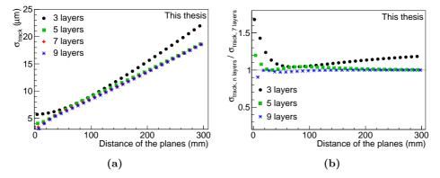
**Figure 4.6:** Effect of the number of layers on the pointing resolution of the tracks. Panel (a) shows the pointing resolution, while panel (b) shows the ratio to the case with 7 planes.
