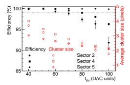
**Figure 5.44:** Comparison of the efficiency and average cluster size results for the different steps of the optimization of the pixels in the sectors of the pALPIDE-3 at  $V_{BB} = -3 V$  and  $V_{CASN} = 105 DAC$  units. The data are taken from Refs. [75, 76].
