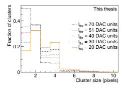
**Figure 5.11:** Example of the cluster size distribution at  $V_{BB}=0$  V and  $V_{CASN}=57$  DAC units for chip W2-25.
