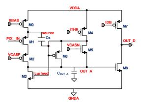
Figure 3.10: Schematic drawing of the practical implementation of the analog frontend in the pALPIDE-1, adapted from Ref. [61].
