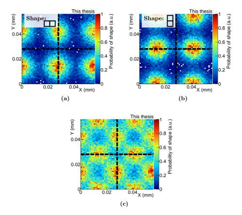
**Figure 5.38:** Probability of the appearance of two-pixel clusters within two times two pixels as a function of the impinging point of the track at  $V_{BB} = 0$  V,  $I_{thr} = 20$  DAC units and  $V_{CASN} = 57$  DAC units for chip W2-25. Panels (a) and (b) show separately the two different rotations indicated on the plot, while (c) shows the two rotations summed up.
