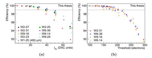
**Figure 5.5:** Detection efficiency values for different chips at  $V_{BB} = 0$  V. In panel (a), the detection efficiency values are shown for the measured chips at  $V_{CASN} = 57$  DAC units as a function of  $I_{thr}$ , while in panel (b), the results are shown as a function of the threshold for all measured  $V_{CASN}$  values for those sensors where the threshold has been determined.
