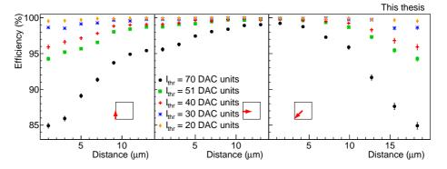
**Figure 5.10:** Detection efficiency as a function of the impinging point of the track along three different paths within one pixel indicated by the drawings. The data are from chip W2-25 at  $V_{BB} = 0$  V and  $V_{CASN} = 57$  DAC units.
