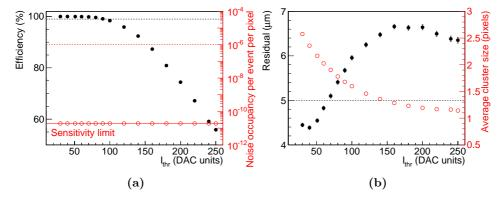
**Figure 5.45:** Panel (a) shows the efficiency and noise occupancy results of the ALPIDE at  $V_{BB} = -3 \text{ V}$  and  $V_{CASN} = 105 \text{ DAC}$  units. The noise occupancy is calculated after masking the ten noisiest pixels. Panel (b) shows the resolution and the average cluster size at the same settings. The data are taken from Refs. [78–80].
