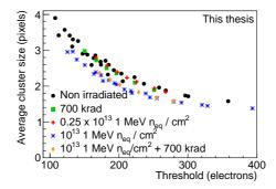
**Figure 5.17:** Comparison of the average cluster size with different irradiation levels for five sensors at  $V_{BB} = 0$  V.
