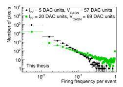
**Figure 5.31:** Distribution of the number of pixels with a certain firing frequency for two extremely low threshold cases at  $V_{BB} = 0$  V for sector 1 of the chip W6-39. In the case with  $I_{thr} = 5$  DAC units and  $V_{CASN} = 57$  DAC units the overall noise occupancy is  $3.1 \times 10^{-3}$  hits/event/pixel, and in the case with  $I_{thr} = 20$  DAC units and  $V_{CASN} = 69$  DAC units, it is  $5.1 \times 10^{-3}$  hits/event/pixel.
