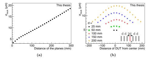
**Figure 4.4:** The pointing resolution at the DUT is shown in two different ways. In panel (a), the distances between the layers are equal and are shown on the x-axis. In panel (b), all the distances are kept at the indicated values (shown by d on the cartoon), but the DUT is moved between the two fixed neighboring planes as indicated on the x-axis, where 0 corresponds to the center between the two neighboring planes.
