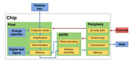
**Figure 3.7:** Schematic drawing of the building blocks of the digital prototypes of the ALPIDE family.
