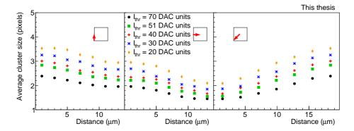
**Figure 5.19:** Average cluster size as a function of the impinging point of the track along three different paths within one pixel indicated by the drawings. The data from chip W2-25 at  $V_{BB} = 0$  V and  $V_{CASN} = 57$  DAC units were used.
