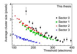
**Figure 5.12:** Comparison of the average cluster size for the different sectors for chip W9-16 at  $V_{BB} = -3$  V.
