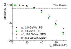
**Figure 5.6:** Detection efficiency values at  $V_{BB} = 0$  V and  $V_{CASN} = 57$  DAC units for the same chip (W2-31) at different momenta and for different particle species.
