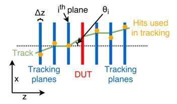
**Figure 4.3:** The drawing illustrates the concept of the tracking.
