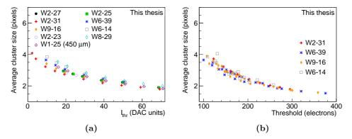
**Figure 5.13:** Panel (a) shows the chip-to-chip fluctuation of the average cluster size as a function of  $I_{thr}$  at  $V_{BB} = 0$  V and  $V_{CASN} = 57$  DAC units, while panel (b) shows it as a function of the threshold at  $V_{BB} = 0$  V for all measured  $V_{CASN}$  values for those sensors where the threshold has been determined.
