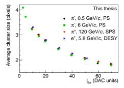
**Figure 5.15:** Average cluster size values at  $V_{BB} = 0$  V and  $V_{CASN} = 57$  DAC units for the same chip (W2-31) at different momenta and for different particle species.
