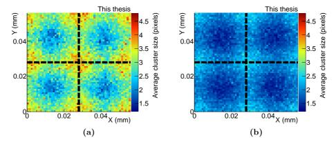
**Figure 5.18:** Average cluster size as a function of the impinging point of the track within two times two pixels at  $V_{BB} = 0$  V and  $V_{CASN} = 57$  DAC units for chip W2-25. Panel (a) shows the cluster size in the case of a low threshold ( $I_{thr} = 20$  DAC units), while (b) shows the same in the case of a high threshold value ( $I_{thr} = 70$  DAC units).
